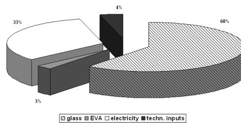
Figure 7: MIPS (abiotic) break-down for frameless CdTe modules
