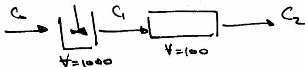
CFSTR  $C_1 = \frac{C_0}{1+kt_0} = \frac{(150)}{1+(10^{-5})(20000)} = \underline{\underline{125 \text{ g/m}^3}}$
