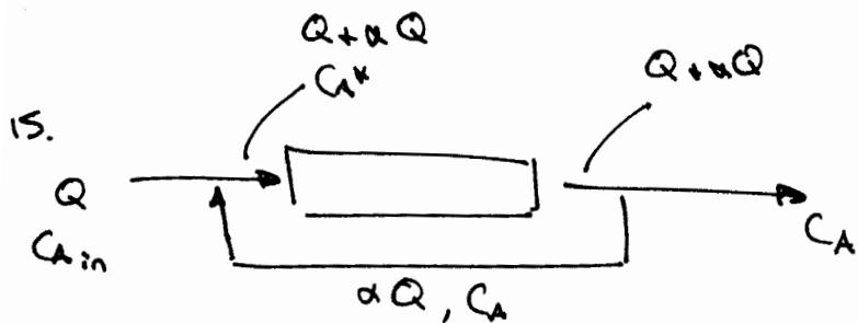
$C_A = C_A^* e^{-kt_0}$  for a 1<sup>st</sup> order rxn @ steady state
