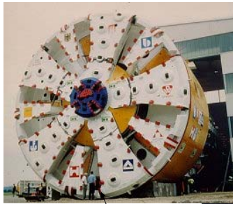
World largest tunneling machine (14.2 m in diameter)
