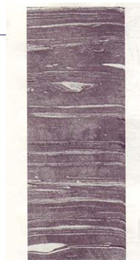
FIGURE 6.25. Two-inch tube sample from flood-plain deposit of Mississippi River near Baton Rouge, La.
