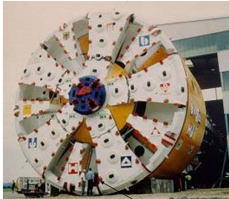
World largest tunneling machine (14.2 m in diameter)
