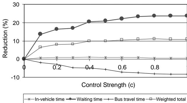
FIGURE 6 Effects of holding control versus control strength.
