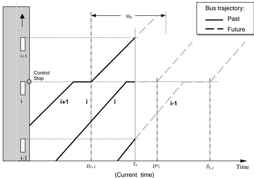
FIGURE 1 Space-time diagram of bus operations.
