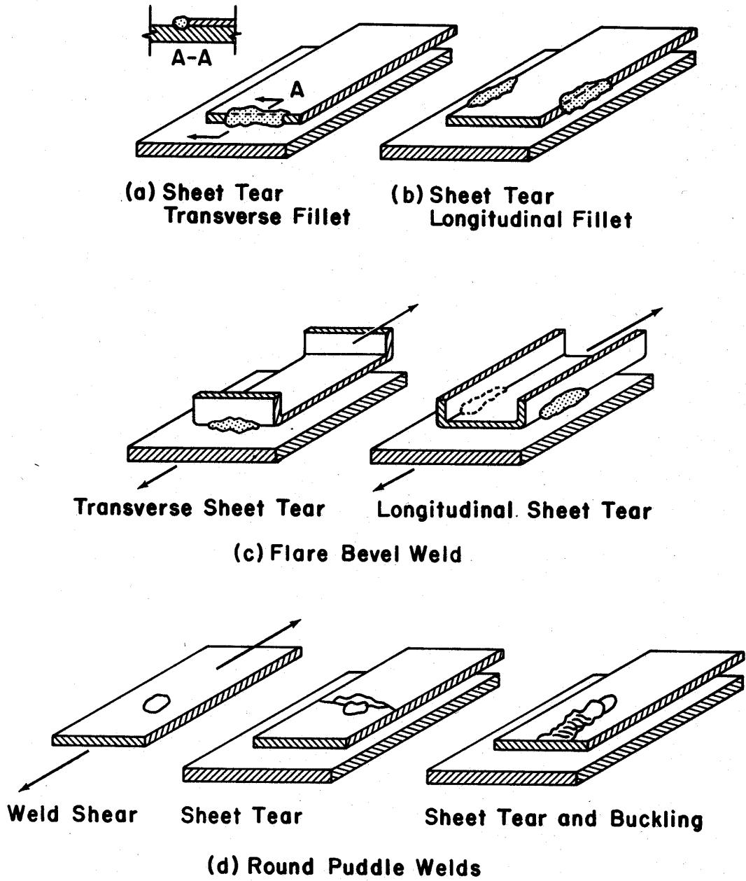
Figure A1 – Typical Failure Modes of Welded Connections
