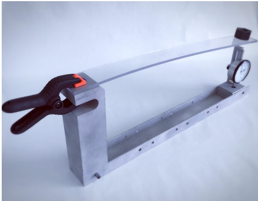
FIGURE 4.3 A Cantilever Beam with an End Load
