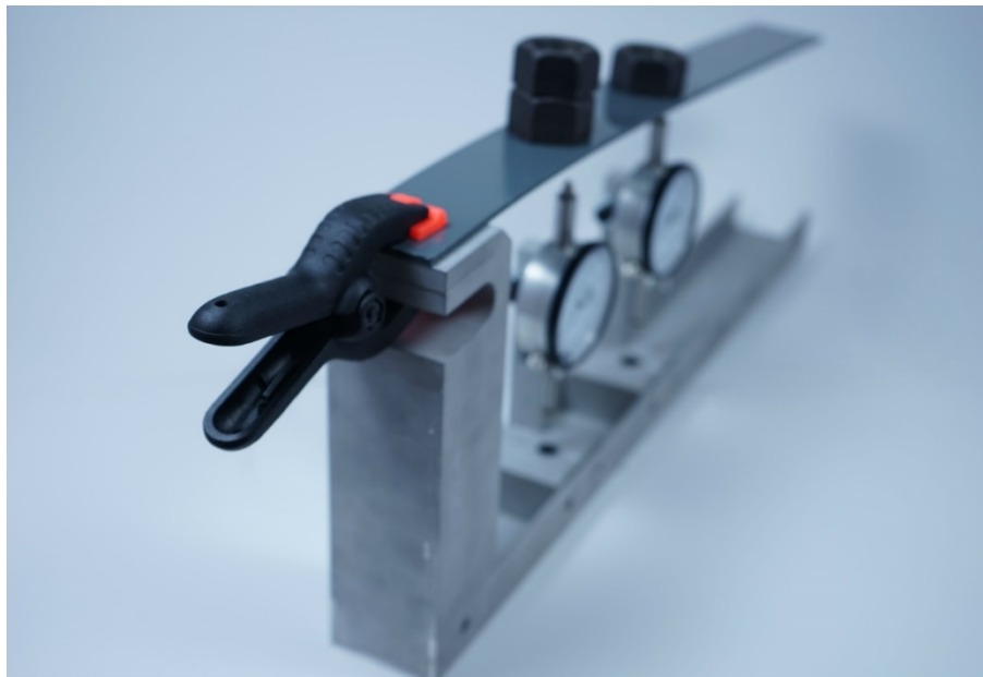
FIGURE 4.1 A Clamped Boundary Condition
