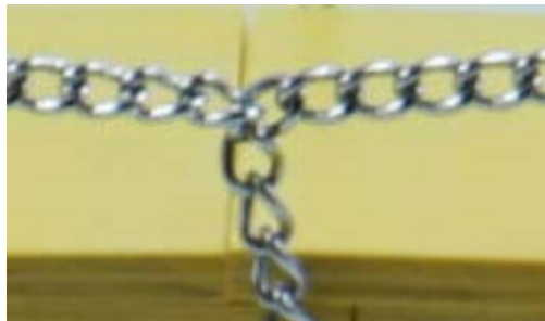
Fig 2 – Detail of Suspender Attachment to Main Chain
