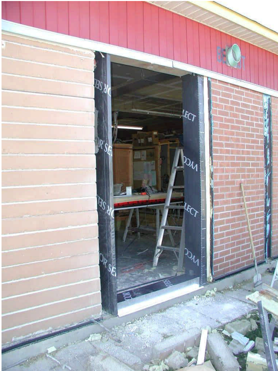
Beghut Ready to Receive a New Test Panel – Note Driving Rain Gauge
