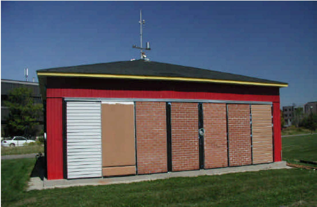
Test House View from South – Vinyl, EIFS, Durisol and Brick clad walls over steel stud, wood stud, and ICF backup are shown in this view
