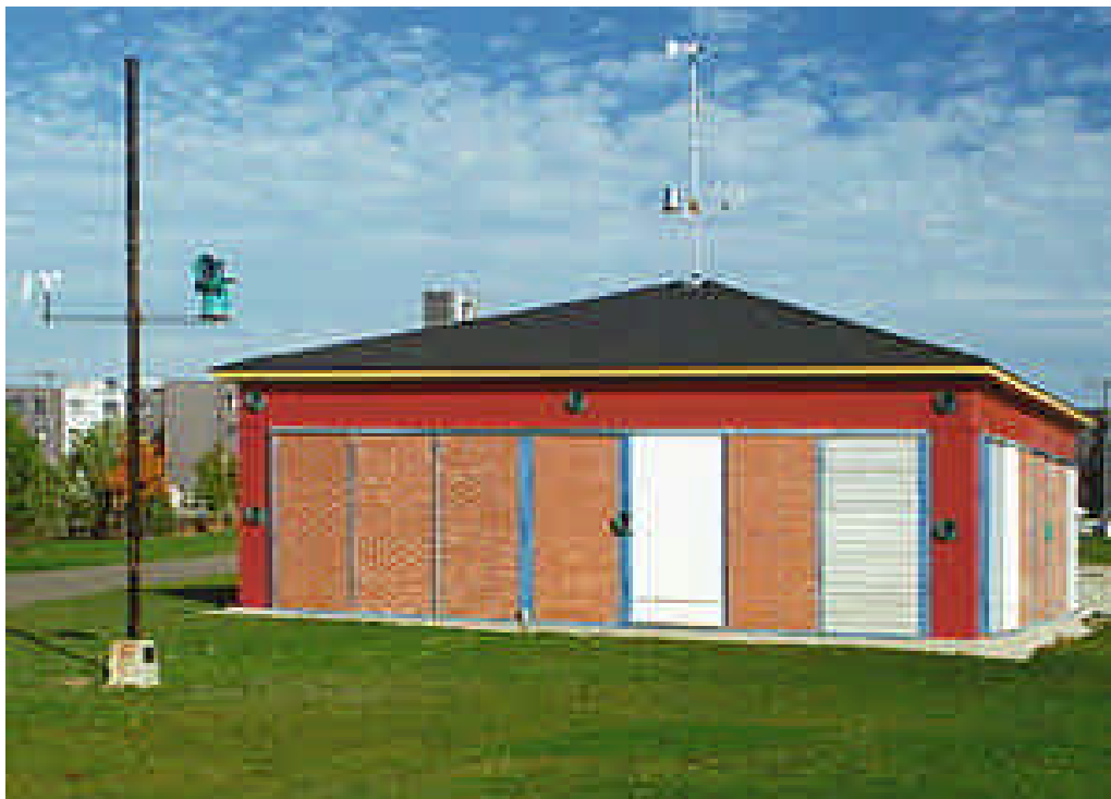
Views of West Face showing Driving Rain Gauges and both Local Weather Towers
