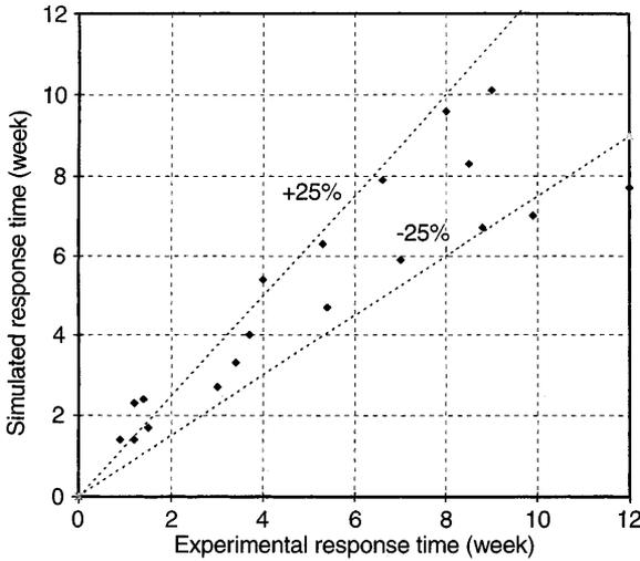
Fig. 7. Comparison of simulated and experimental response times needed for visual appearance of mould growth on spruce sapwood in constant conditions
