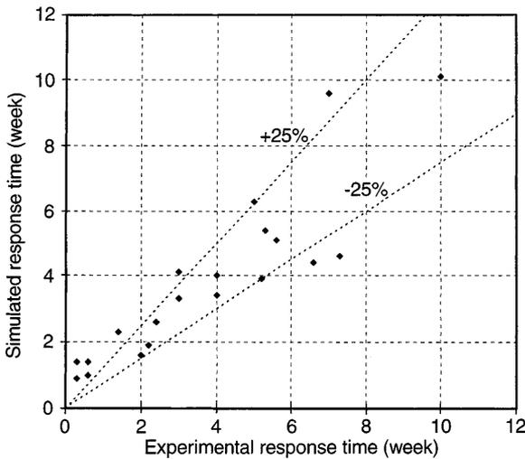
**Fig. 6.** Comparison of simulated and experimental response times needed for initiation of mould growth on spruce sapwood in constant conditions
