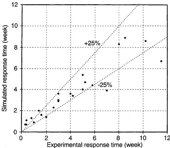
Fig. 4. Comparison of simulated and experimental response times needed for initiation of mould growth on pine sapwood in constant conditions
