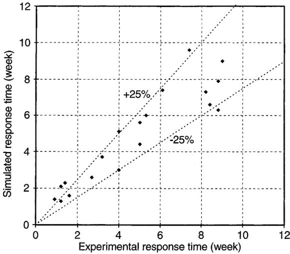
**Fig. 5.** Comparison of simulated and experimental response times needed for visual appearance of mould growth on pine sapwood in constant conditions
