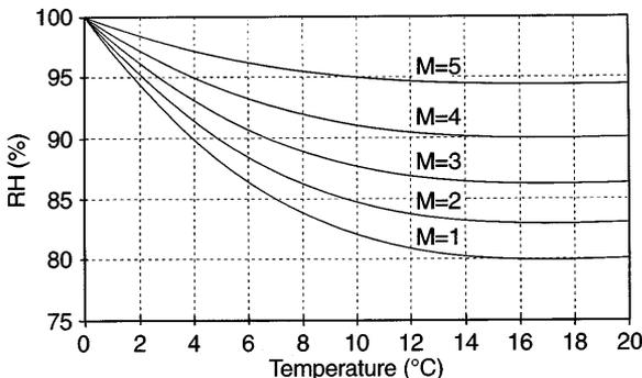
Fig. 2. Temperature-dependent critical relative humidity needed for mould growth at different values of mould index
