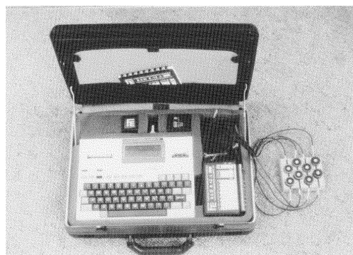
Figure 6.1 Daylighting Data Acquisition System (Courtesy: Fowlkes Engineering).
