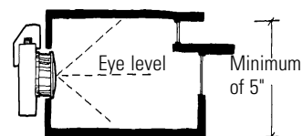
Figure 5.10 Position of camera inside model
