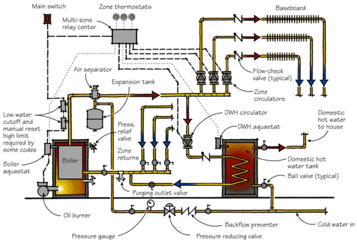
**Figure: Typical Baseboard Hydronic Installation (from another article)**
