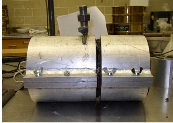
Figure 2. The shear tube test - three point loading
