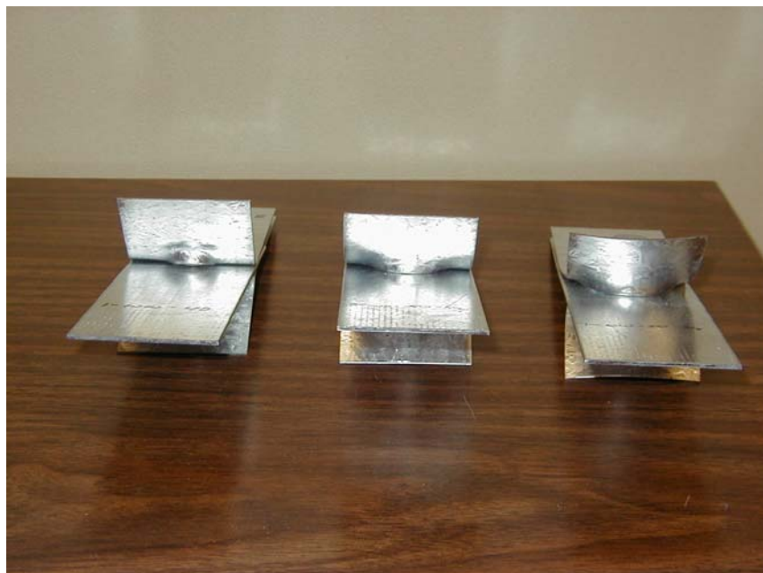
Figure 10: Failed Double Shear Specimens With Washers
