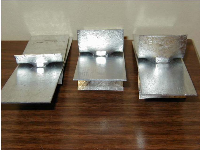
Figure 9: Failed Double Shear Specimens Without Washers
