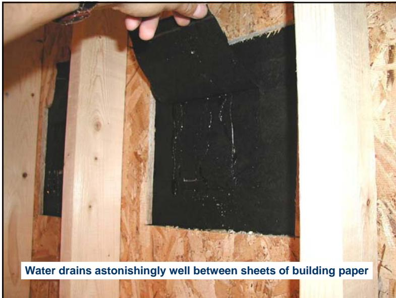
Water drains astonishingly well between sheets of building paper
