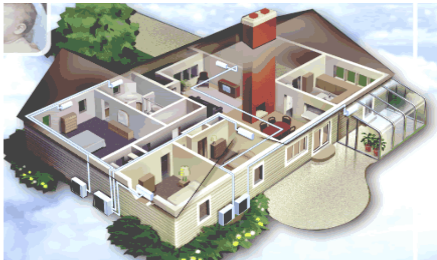
Ductless Split Systems use a refrigerant, not air, to transfer heat and cool.
